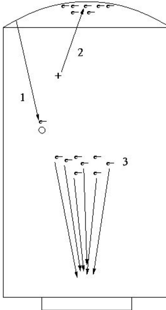
As well as ion feedback, clusters are present due to effects such as micro-discharges, where dielectric breakdown of the air causes flashes of light. Also, errors in reading in the data from the L1 boards if the read/write pointers get out of step, etc, can cause clusters of hits
